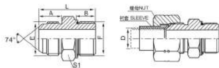
美制JIC外螺纹74°外锥/英管外螺纹O形圈 JIC MALE 74° CONE/BSP MALE O-RING
